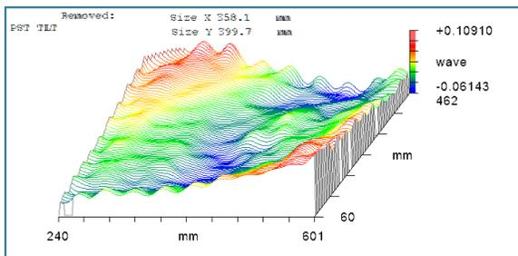
Single-pass wavefront measurements at 1054 nm: P-V 0.171 Wave, rms 0.031 wave
